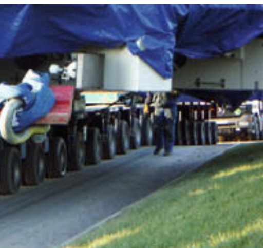
Special transporter with 22 axles for the 212 tons generator of the E-112
