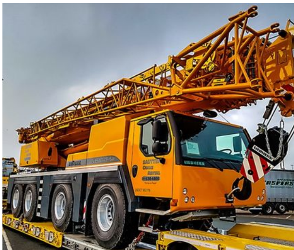
The LTM1090-4.2 has a longer chassis but similar turning circle
